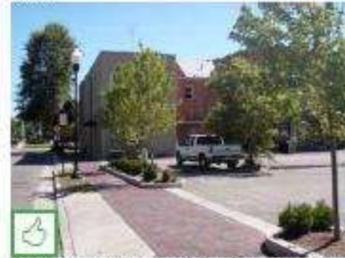
This parking access apron appropriately places the priority on pedestrians by continuing the sidewalk uninterrupted across the driveway.
